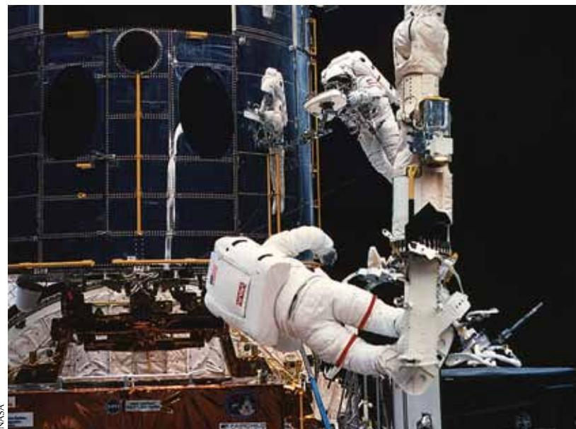
Anchored on the end of orbiter Endeavour's remote manipulator system arm, astronaut Jeffrey Hoffman (foreground) prepares to install the new wide field planetary camera into the empty cavity of the Hubble Space Telescope (HST). Astronaut Story Musgrave works with a portable foot restraint.
